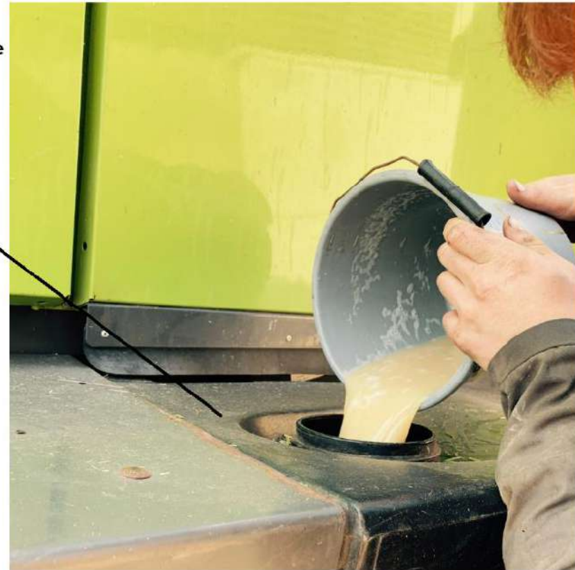
Chopper with a silage additive tank and dosing system
